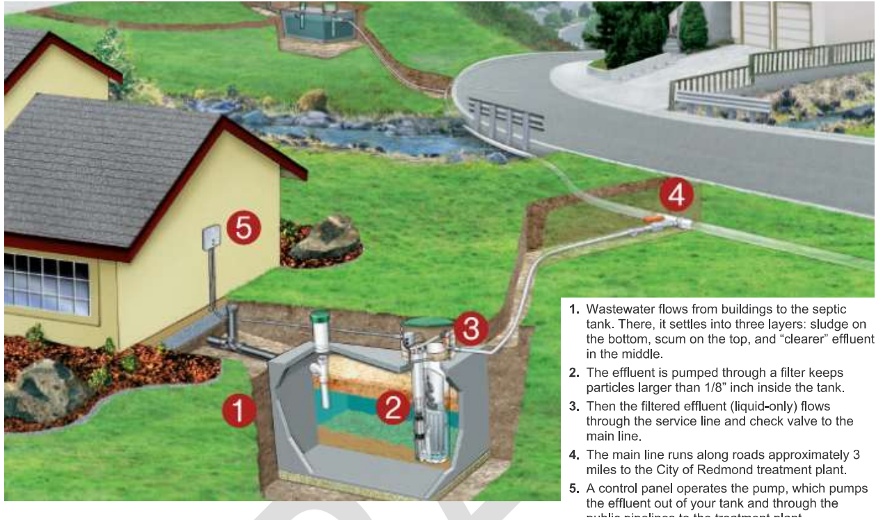
Figure 32 Typical Onsite Residential STEP System Components
