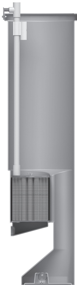
PVP-Series Pump Vault, cross-sectional side view
